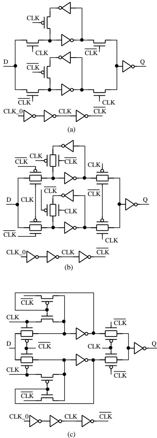
FIGURE 2 (a) The design of CMOS DET flip-flop in Ref.[7];
