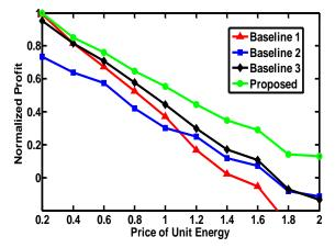
**Figure 3:** The normalized total profit versus the unit energy price of the proposed near-optimal algorithm and three baseline algorithms.
