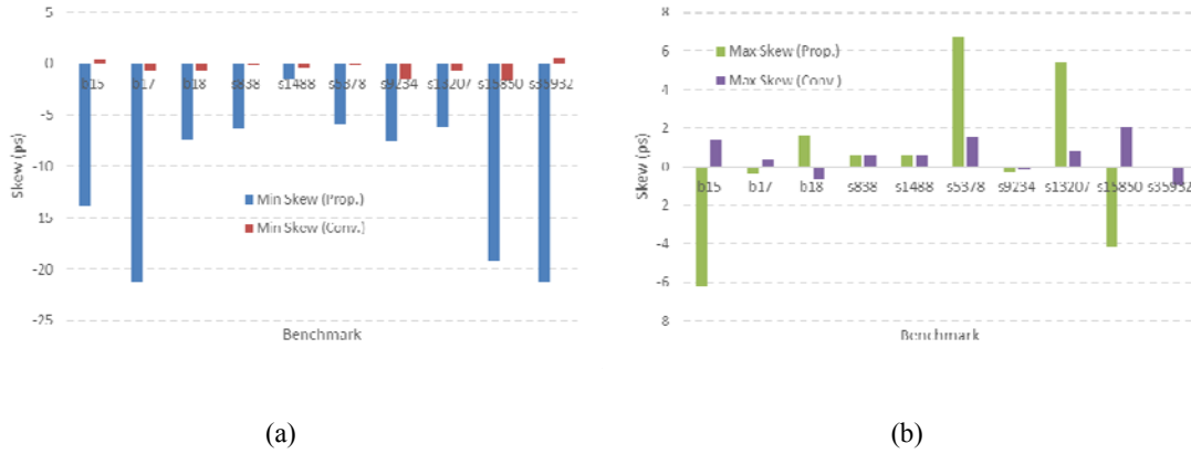
Figure 9. a) Minimum and b) Maximum Clock Skew for both CSAM and Conventional NBTI Mitigation Techniques.
